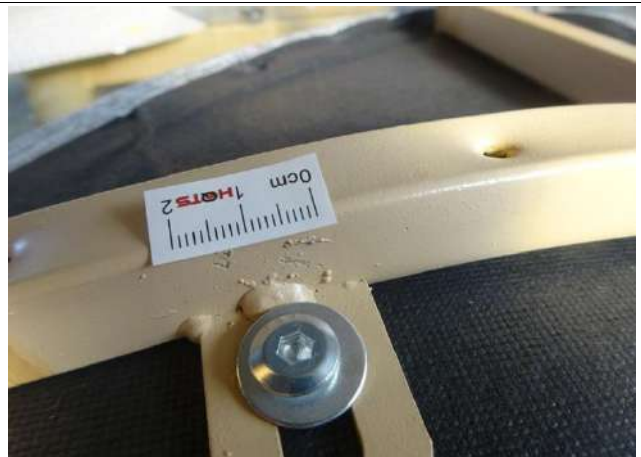
Dining Chair Defect-Scratched mark at leg(1.5cm)-mi
