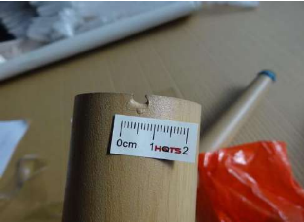
Dining Table Defect-Broken at leg(0.6cm)-ma
