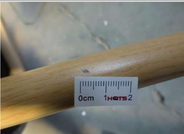
Dining Chair Defect-Scratched mark at leg(0.5cm)-mi
