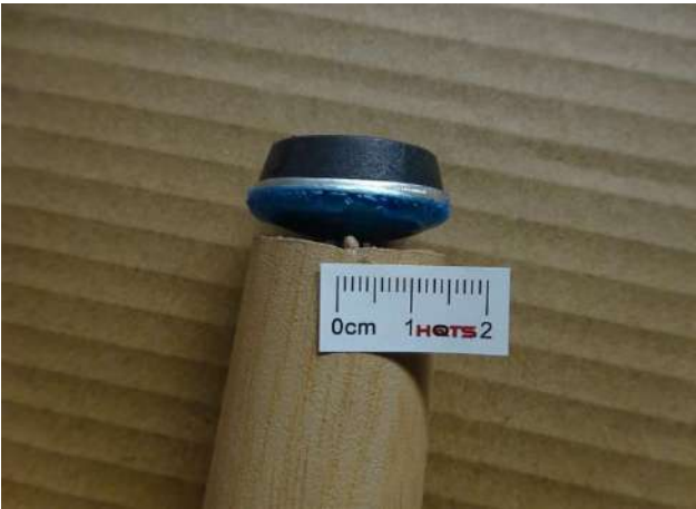
Dining Table Defect-Convex mark at leg(0.3cm)-mi
