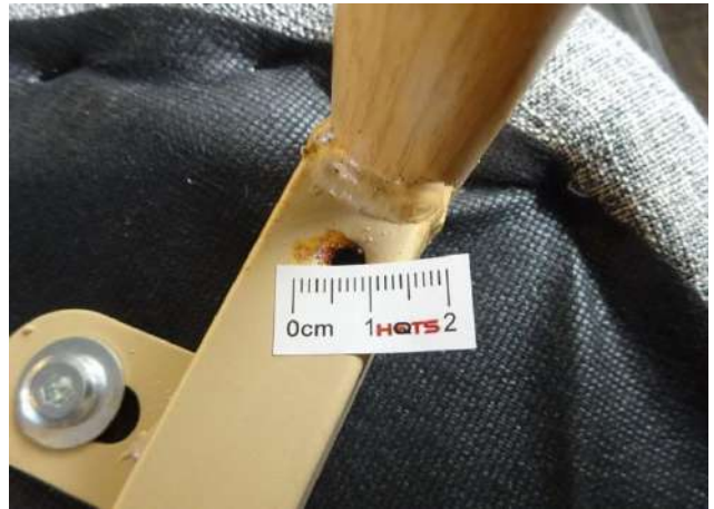
Dining Chair Defect-Rusty mark at hole(1cm)-ma
