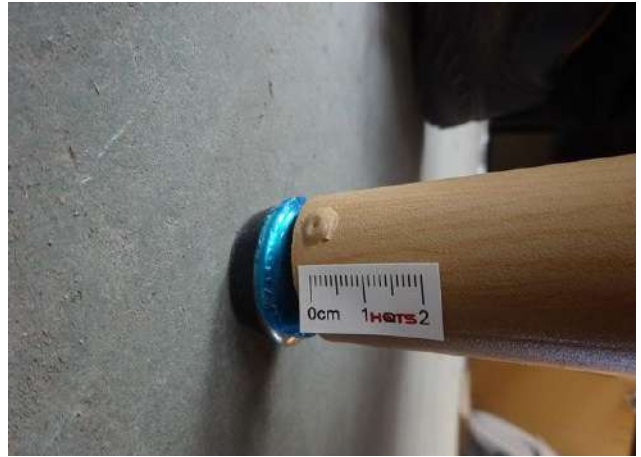
Dining Table Defect-Convex mark at leg(0.5cm)-mi
